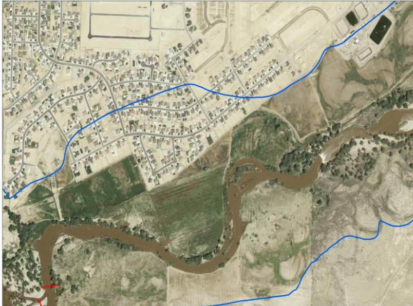
River Park Subdivision and Park/Trail Project Blue line denotes the FEMA 100-year floodplain zone
